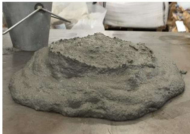
Images 5 and 6. Samples of “Monte Morello” and “Sillano” soils conditioned with Polyfoamer ECO/100.
