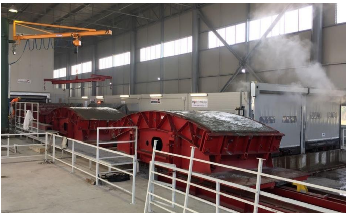
Images 2 and 3. Segment production with Dynamon NRG1015S and one of the niches waterproofed with Mapeplan TU20.
