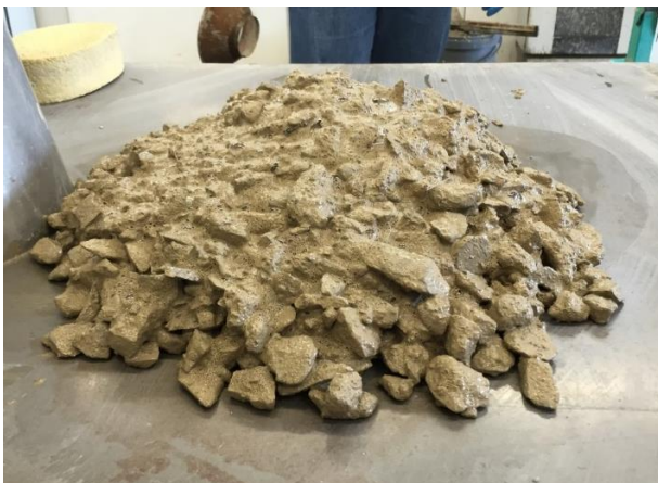
Images 5 and 6. Samples of “Monte Morello” and “Sillano” soils conditioned with Polyfoamer ECO/100.
