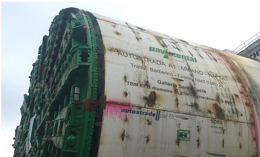
Image 1. 15.96m TBM diameter: the largest TBM ever used in Europe and one of the largest in the world.
